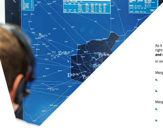
As it is difficult to judge for both pilots and ATCOs whether an aircraft is on the right glide path, the last phase of the sequencing can easily result in **unpredictable and expensive level flight in low altitudes**.
